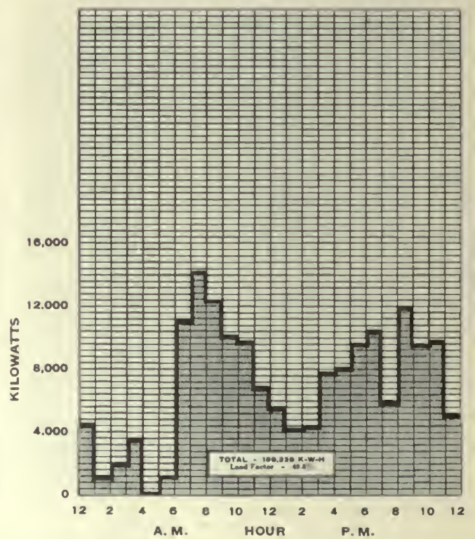
FIG. 603. ENERGY CHART. Kilowatt-Hours at the Pantograph for the Average October Day for 11,000-Volt A. C. Operation, Through Passenger Service.
